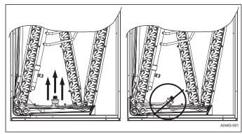
FIGURE 9: Recommended Distributor Adjustment
