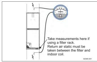
FIGURE 18: Duct Static Measurements
