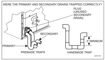
FIGURE 19: Drain Traps
