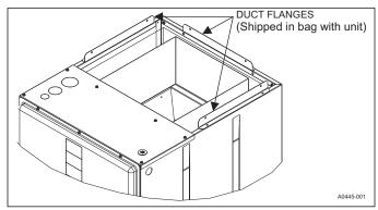
FIGURE 7: Duct Attachment
