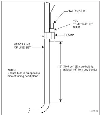
FIGURE 14: Vertical Temperature Bulb Orientation
