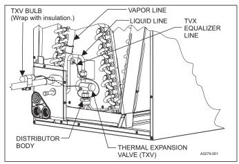
FIGURE 12: TXV Bulb and Equalizer line Installations
