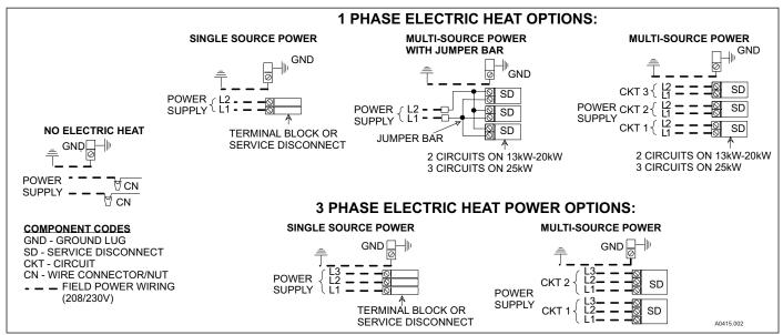
FIGURE 16: Line Power Connections
