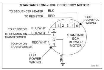
FIGURE 17: Blower Speed Connections
