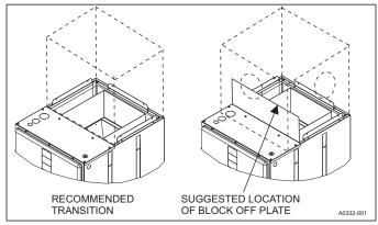
FIGURE 8: Duct Work Transition
