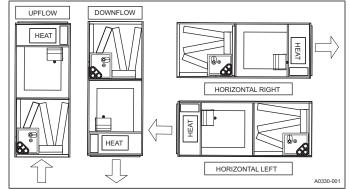
FIGURE 4: Typical Installation
