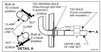
FIGURE 13: Proper Bulb Location
