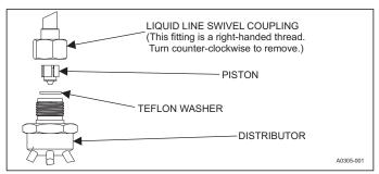
FIGURE 10: Piston Installation
