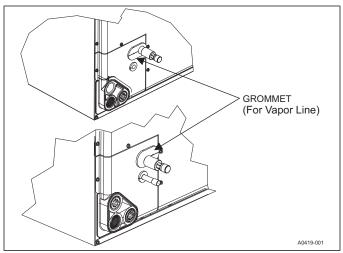
FIGURE 15: Vapor Line Grommet
