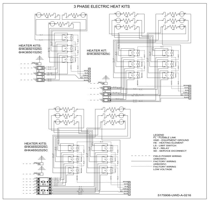
FIGURE 22: Wiring Diagram - Three Phase Heat Kits 208-230V
