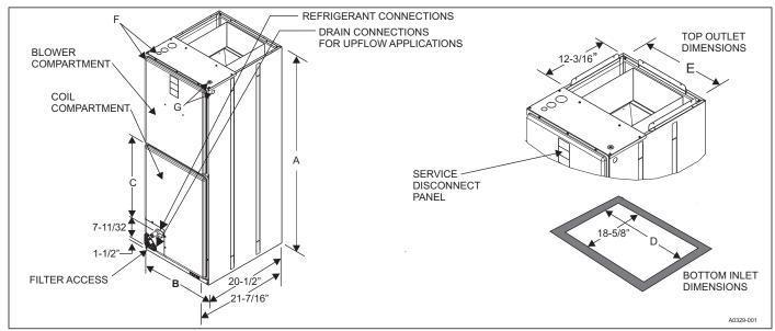
FIGURE 3: Dimensions & Duct Connection Dimensions
